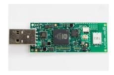
The AL5630 implements a bridge between the AL5704 and the RJ45 Ethernet interface. The AL5630 is shown in the following image.
