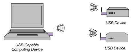
Connection of multiple radios simultaneously requirs a Wireless USB device driver on the computing device. This case also requires the purchase of multiple evaluation kits.
