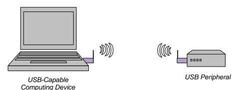
Most single USB peripheral devices may be connected without the need for a Wireless USB device driver on the computing device.
