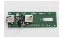
The AL5704 plugs into the AL5619's USB2.0 type A jack in the center of the adapter board. The USB peripheral, composite, or hub is connected to the USB2.0 type A jack on the edge of the board using an appropriate USB cable (the same cable that would be used for plugging the USB device into a computing device). The AL5619 accepts a 5V power supply which powers the radio and the downstream USB device.
