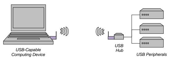
The wireless connection of a USB hub requires a Wireless USB device driver on the computing device.
