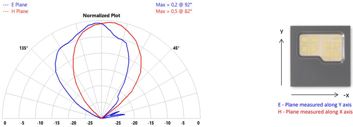
Figure 18 Combined Radiation Pattern Measurements of TX and RX Patch Antennas
