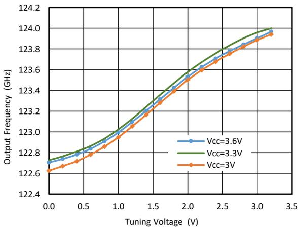
Figure 12 VCO Pushing -  $V_{cc} \pm 300\text{ mV}$
