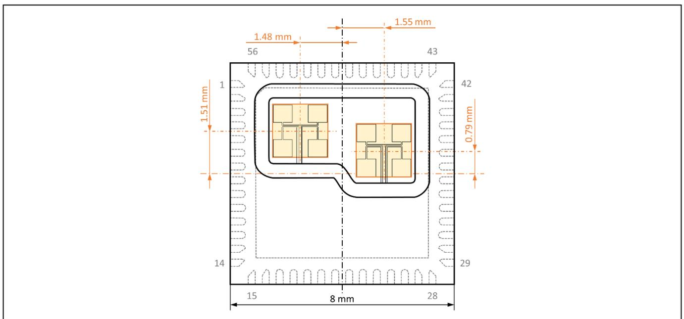
Figure 4 Antenna Position (top view)
