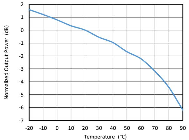
Figure 17 Output Power Swing vs. Temperature (Normalized to 20°C)
