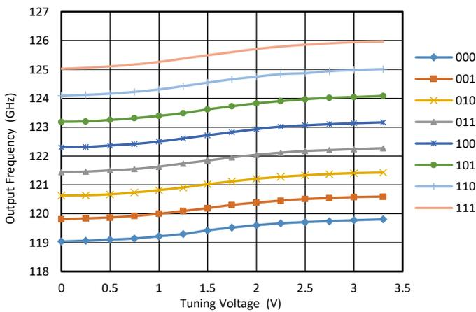
Figure 10 VCO Tuning Curves.  $V_{t0}$  is varied, while  $V_{t1}$ ,  $V_{t2}$  and  $V_{t3}$  are driven high or low. For example, 011 means  $V_{t3} = 0$ ,  $V_{t2} = 3.3\text{ V}$ , and  $V_{t1} = 3.3\text{ V}$ .
