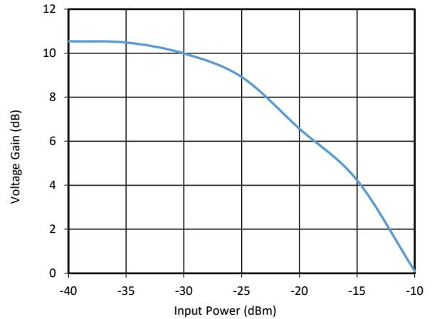
Figure 9 Measured Conversion Gain of the Receiver
