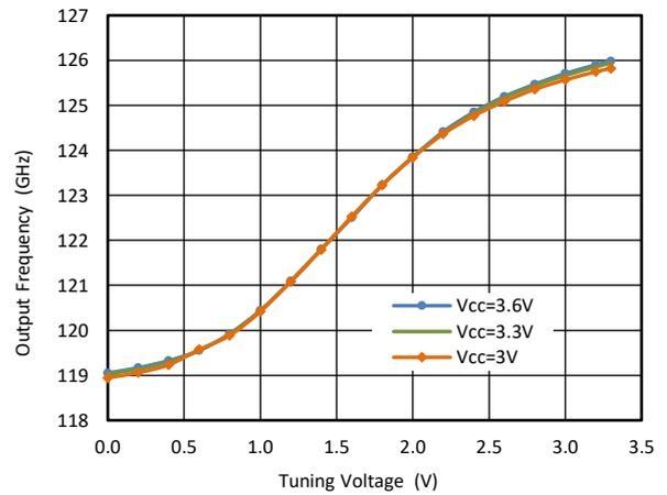
Figure 15 VCO Pushing - Full Bandwidth Operation. All tuning voltages,  $V_{t0} = V_{t1} = V_{t2} = V_{t3}$
