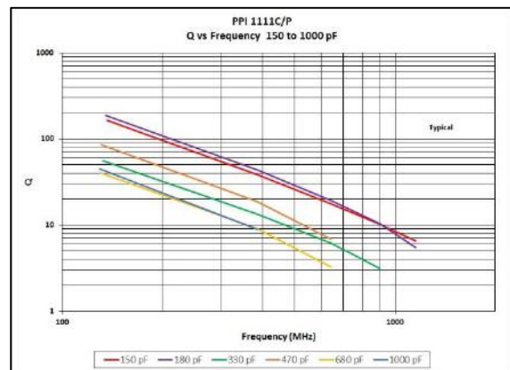
1111C Q vs Capacitance
