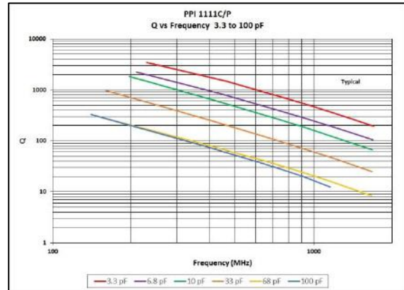
1111C/P Q vs Capacitance
