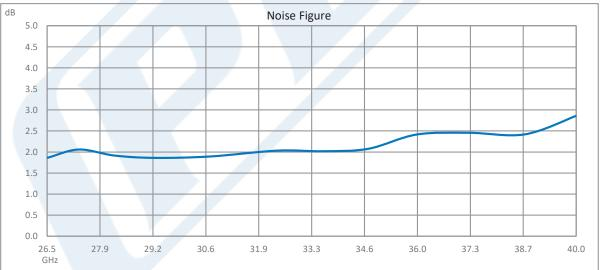
Click the following link (or enter part number in "SEARCH" on website) to obtain additional part information including price, inventory and certifications: Ka Band Low Noise Amplifier, 26.5 GHz to 40 GHz, 35 dB Gain, 2.5 dB Noise Figure, 12V, 2.92mm PE15A63021
