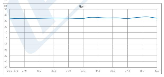
Click the following link (or enter part number in "SEARCH" on website) to obtain additional part information including price, inventory and certifications: Ka Band Low Noise Amplifier, 26.5 GHz to 40 GHz, 35 dB Gain, 2.5 dB Noise Figure, 12V, 2.92mm PE15A63021
