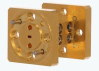
Farran's BPF-06-0003 is a high performance waveguide band-pass filter offering low in-band insertion loss, high out-of-band rejection and excellent input and output match. Suitable for use in communications equipment, radar systems and millimeter-wave instrumentation.
