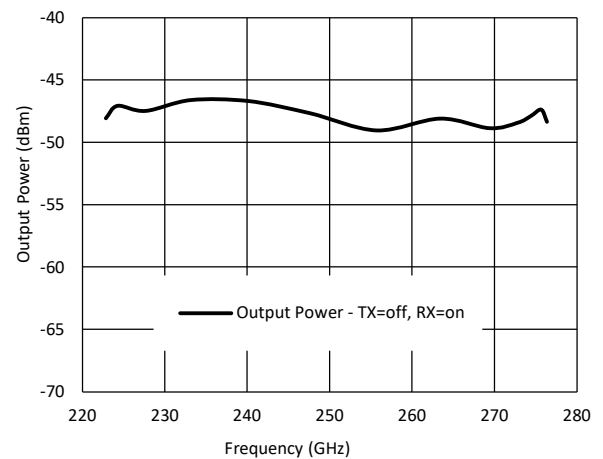
Figure 16 Output power measured at antenna input with internal VCO, TXEN=0V, TXpwr=0V.
